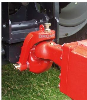
*Figure 14: Image of ‘ball and spoon’ type coupling.
