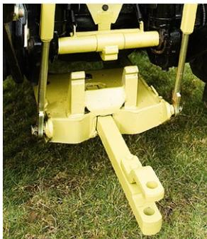
*Figure 13: Image of ‘pin and eye’ type coupling.
