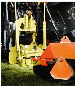
*Figure 12: Image of ‘hook and ring’ type coupling.
