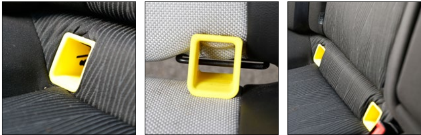
ISOFIX connection points in the back seat (Some are not clearly marked, so you should consult your car manual for advice in this case.)
