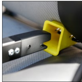
Plugging in the ISOFIX connectors into the connection points
