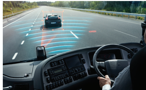
Example of Adaptive cruise control.
