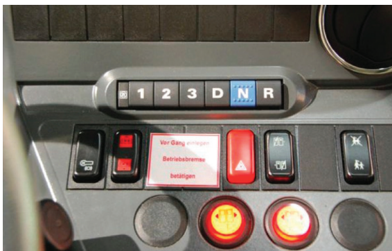
Example of ZF automatic transmission.
