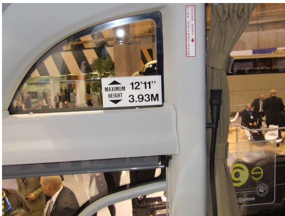
Example of vehicle overall height warning sticker.
