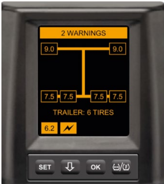
Example of tyre system warning
