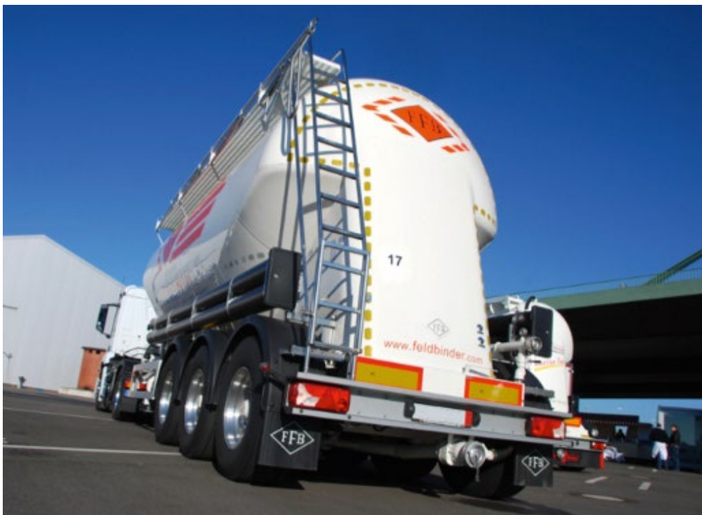
Example of elevated catwalk
