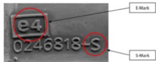
Figure 2: E-Mark and S-Mark on tyre sidewall
