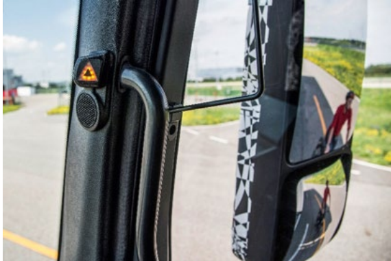
Example of cyclist detection system
