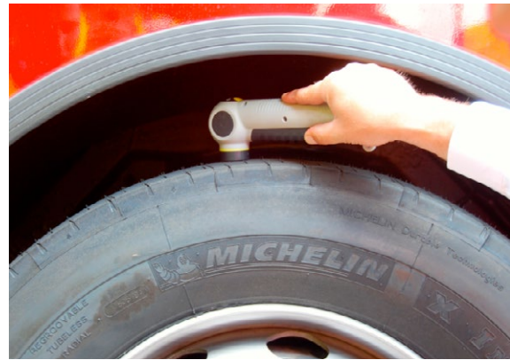
The instrument shown above is a RFID (Radio Frequency Identification Disc) scanner, which can check the tyre location, pressure and tread wear
