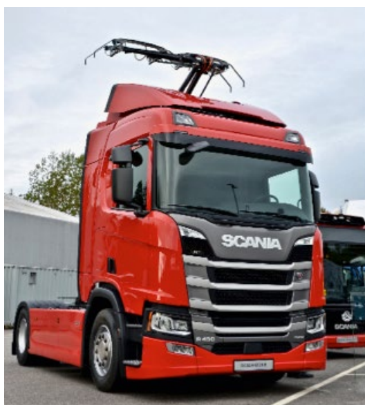
Example of electrically powered truck. Note the recharging mechanism on the roof which retracts when charging is completed.
