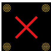
Tunnel Lane Closed
