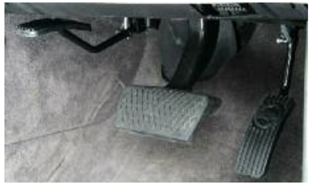
Twin flip accelerator – Brig Ayd
