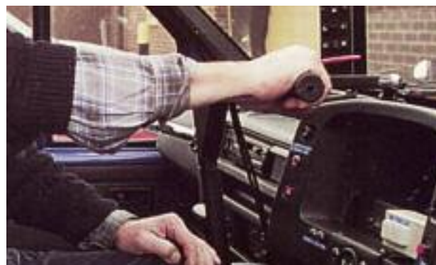
One hand tiller from Jim Doran – you twist the grip to accelerate and squeeze the lever to brake
