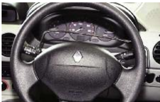
This rod transfers the indicators from one side of the wheel to the other, so you can operate the indicators with your right hand – Alfred Bekker
