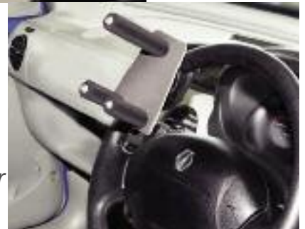
The glove has a sleeve that fits over a peg on the steering wheel
