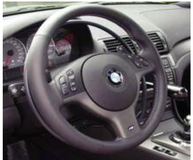
K5 under ring from Autoadapt – push or pull on the ring to accelerate
