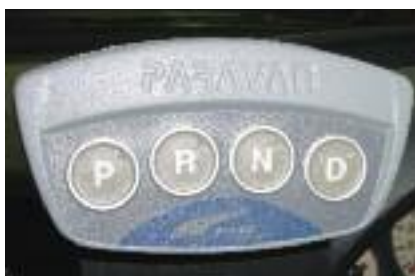
Spacedrive push-button gear selector – Adaptacar
