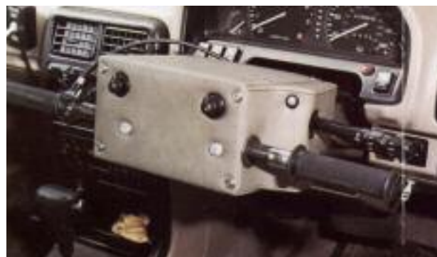
The two handed tiller from Jim Doran also controls speed – you twist the handle to accelerate and push the tiller forwards to brake
