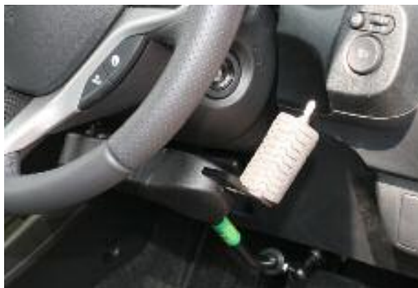
Indicator switch on hand controls – this one is from Jeff Gosling
