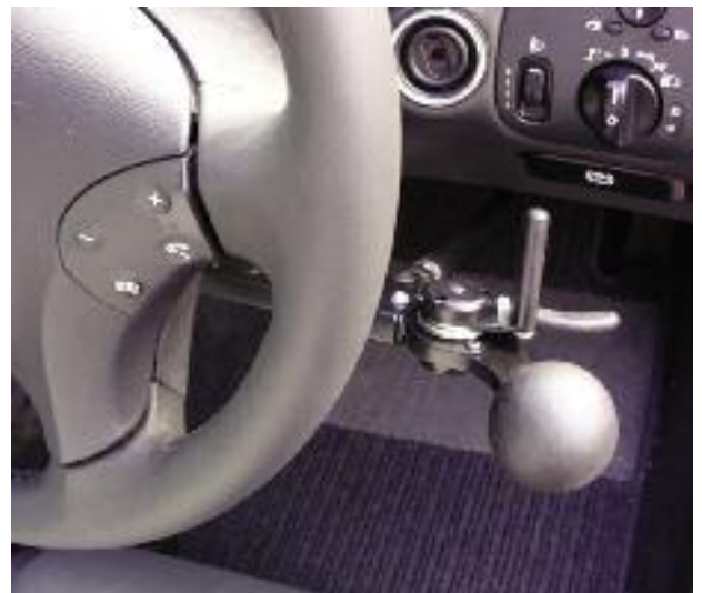
Brig Ayd Trigger control. Pull trigger to accelerate (electronic), push away to brake
