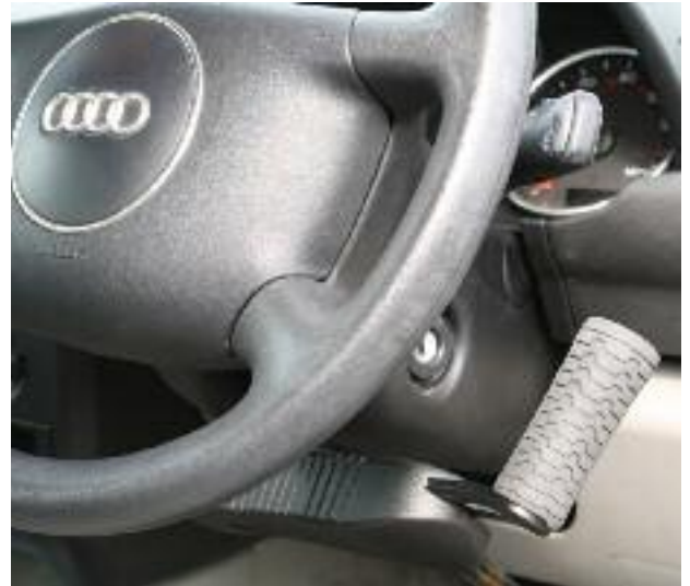
Jeff Gosling push/pull hand control. Pull to accelerate, push to brake
