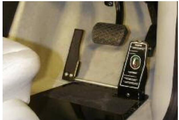
Quick release accelerator – Brig Ayd
