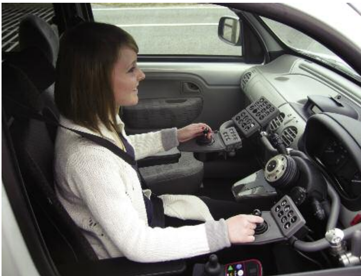
Drive from wheelchair vehicle with joystick steering and speed control; keypads for gears and secondary controls
