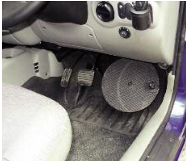
Foot steerer from Bristol Street Versa - turntable used with an adapted shoe
