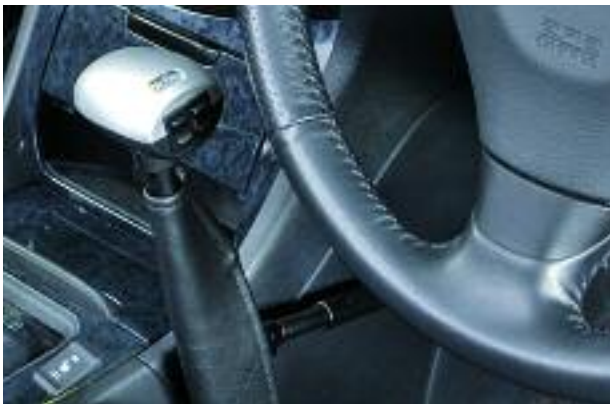
Control switches on floor mounted hand control (Carospeed from Autoadapt)
