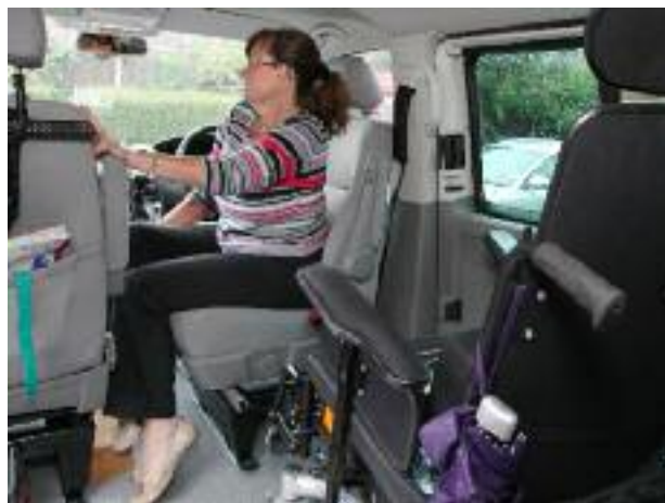
A swivelling seat allows easier access from a wheelchair
